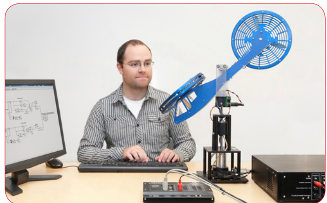
2 DOF Helicopter workstation
