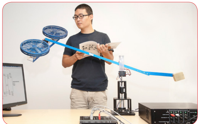
3 DOF Helicopter workstation
